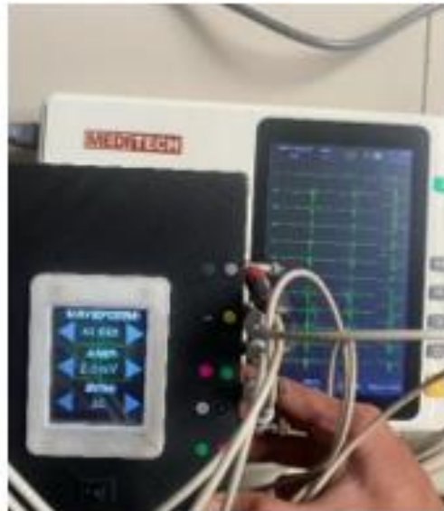
Figure 5. The signal shape produced from the tool setting at 30 BPM.
