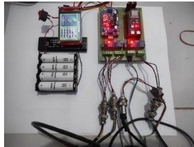
Figure 7. Prototype PCB design
