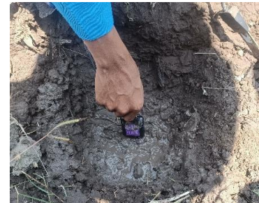
Figure 8. Installation of sensors in soil samples.
