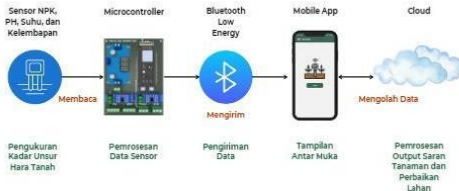
Figure.4. Installation and Working Principle of Soil Nutrient Monitoring Equipment.
