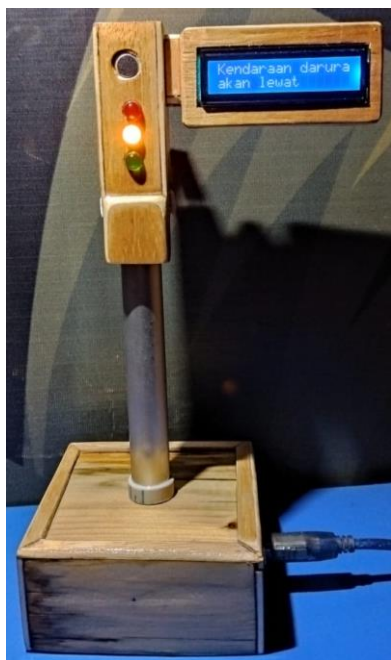
Gambar 7. Purwarupa Smart Traffic Light
